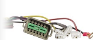
(2) 12 Pin Deutsch Connector & (3) 2 Pin Mini-Fit™ Molex
